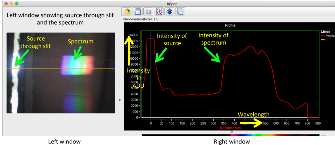
Figure 7: Intensities of light source and spectrum from RSpec Explorer software.
