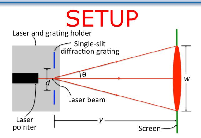
d – width of slit y – distance of screen from slit w – width of light blob  $\theta$  – angle of diffraction
